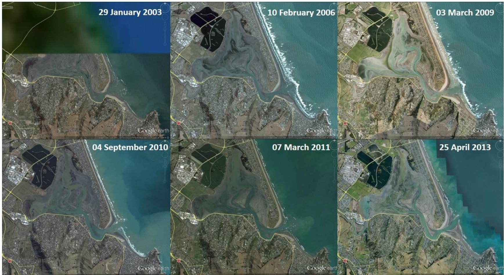
Figure 4-10 Time series of Google Earth images of the inlet ( 43^{\circ} 33' 41.45''\text{S} , 172^{\circ} 45' 14.44''\text{E} ) and the estuary from 29 January 2003 to 25 April 2013. For direct comparison of the inlet and estuary morphology, it has to be considered that the images have not been referenced to the respective tidal phases yet.
