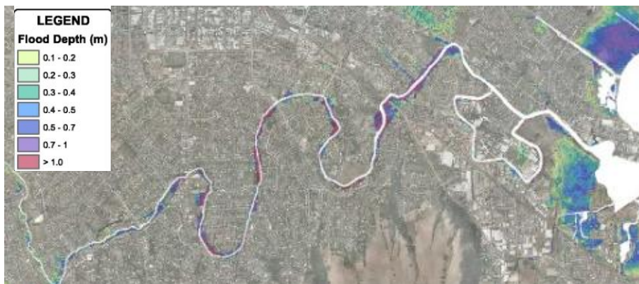
Figure 5-1 Heathcote River area: (a) impacts of tectonic uplift (Tonkin & Taylor, 2013); (b) pre-100 year annual return interval (ARI) event flood depth; and (c) post 2010-2011 earthquake sequence ARI event flood depth excluding stop-banks and climate change (Tonkin & Taylor 2013).
