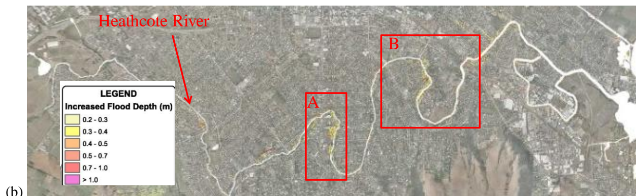
Figure 5-2 Heathcote River: (a) cumulative elevation change along the river pre-2010 to post June/December 2011 (Tonkin & Taylor Ltd, 2013, Figure A10); (b) overland flow increased flood depths post-December 2011 compared to pre-September 2010 (Tonkin & Taylor, 2013).
