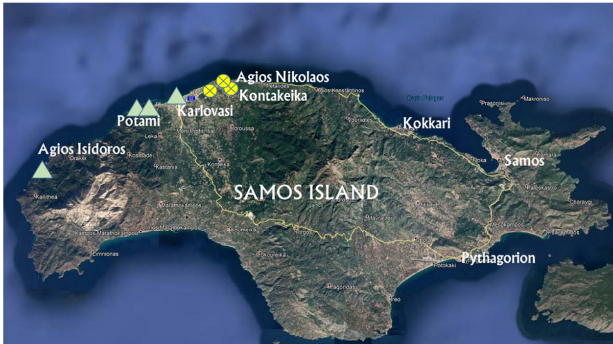
Figure 1.31. Google Earth map of Samos Island: Green triangles correspond to permanent uplift and yellow circles to surface ruptures (Lekkas et al., 2020).
