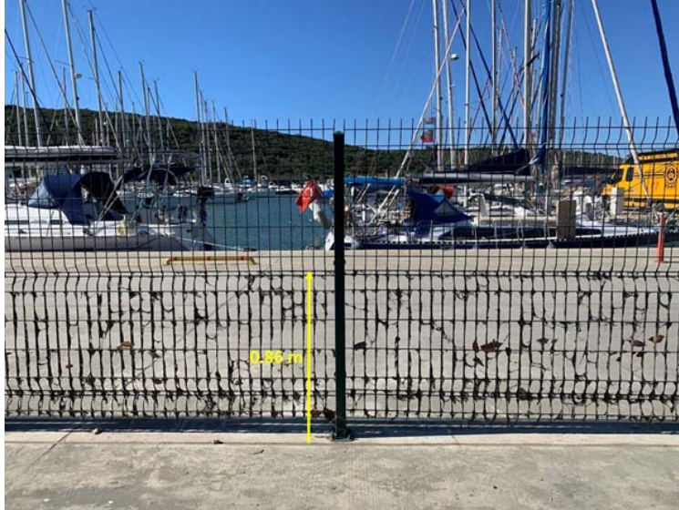
Figure 2.13. Tsunami traces on the garden fence of Teos Marina corresponding to a flow depth of 0.86 m. Classic presentation of debris “escalator” showing maximum flow depth.
