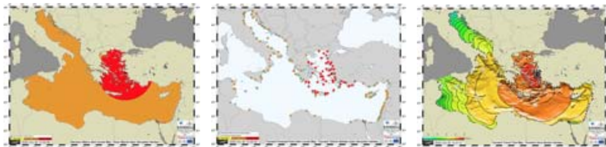
Figure 2.36. Enhanced products disseminated by KOERI-TSP during the 30 October 2020 11:51 UTC M7.0 Samos-Aegean earthquake. Threat Level Zones Map (left), TFP Threat Level Map (center), Tsunami Travel Time Map (right).
