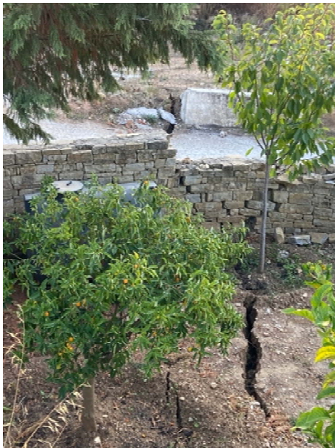
Figure 5.30. Ground and pavement cracks in the village of Kontakeika (Samos), indicative of the mobilization of an extended but mild slope or more broadly characterized as seismically-induced secondary ground failures. The cracks extended on both sides of the street through soft soil formations.
