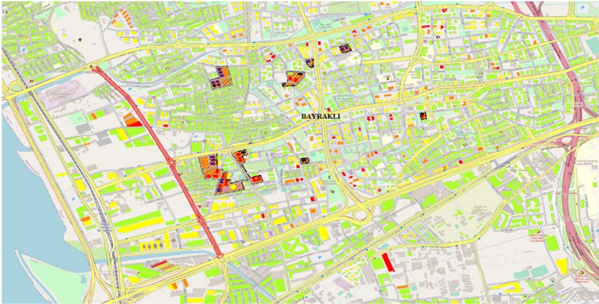
Figure 7.4. Damage distribution in the Bayraklı district of Izmir (green, yellow, orange and red colors indicate buildings with no, slight, moderate and heavy damages, respectively. The black and pink indicators show the buildings that have totally or partially collapsed during the earthquake)
