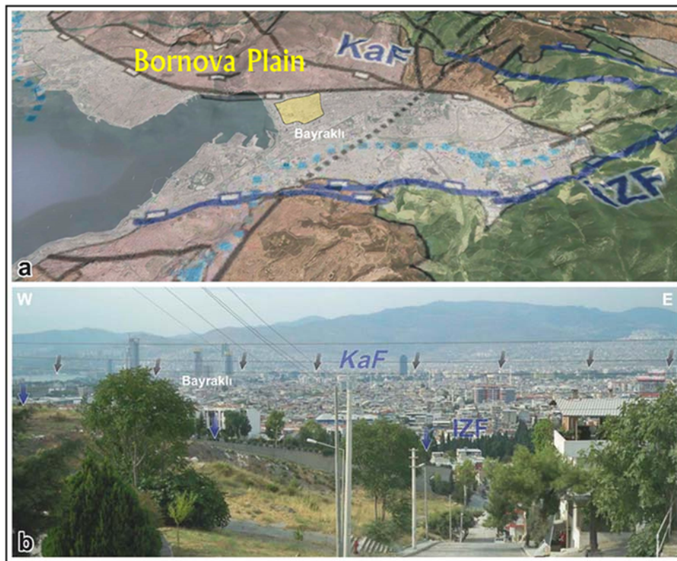
Figure 1.5. Upper: satellite view of İzmir Bay with geology (Uzel et al., 2013). Lower: a field photo of faults bounding İzmir Bay. KaF: Karşıyaka Fault, IZF: İzmir Fault. Historical seismicity shows that damaging earthquakes occurred near the broader İzmir metropolitan area.
