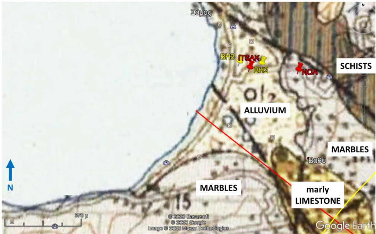
Figure 4.28. Detail of geological map of the area of the two recording sites (ITSAK and NOA) at Vathy, as well as locations of two available boreholes (BH3 and BH2); Geological info from HSGME (1979) map.
