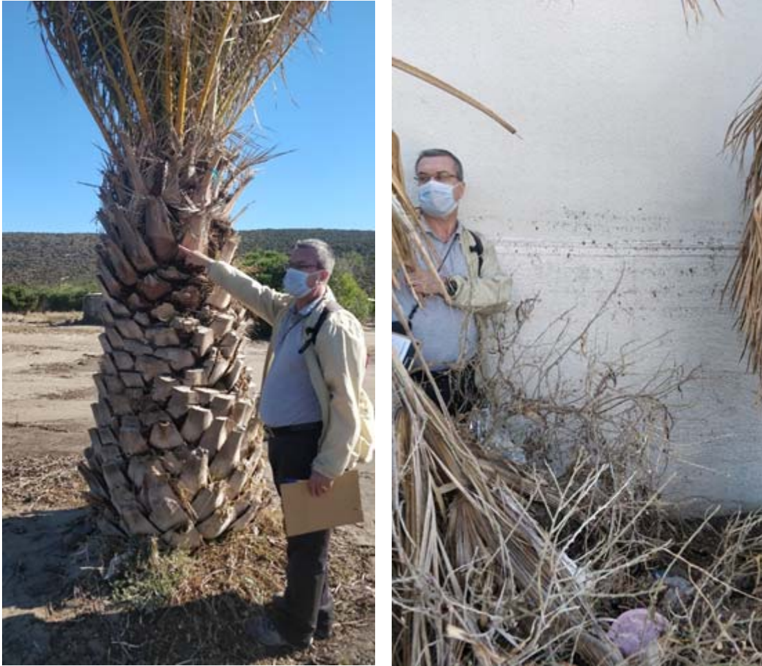
Figure 2.7. (Left) Wave traces on the palm tree (1.90 m) near the coastline (38.19600N 26.48859E), and (Right) trace of debris materials accumulated at the outer wall (1.50 m) of a house (38.19587N 26.49027E).
