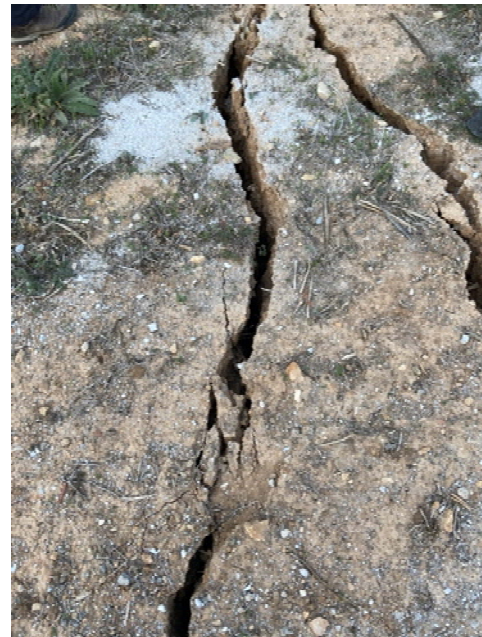
Figure 5.30. Ground and pavement cracks in the village of Kontakeika (Samos), indicative of the mobilization of an extended but mild slope or more broadly characterized as seismically-induced secondary ground failures. The cracks extended on both sides of the street through soft soil formations.
