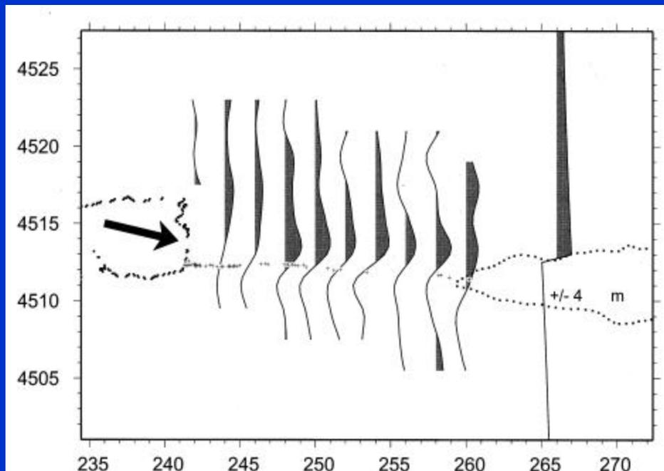
Slip distribution from Kocaeli earthquake using 20-m resolution SPOT data (Fiegel et al. 2002, BSSA)
