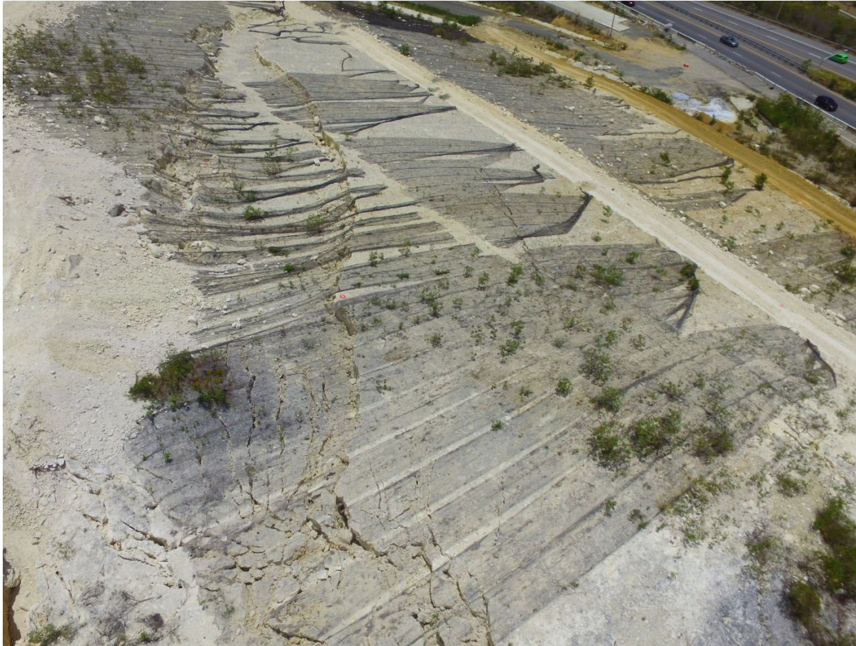
Figure 2-15: Aerial image showing pre-Maria condition of preexisting landslide at PR-9 north of Ponce (Lat: +18.033145, Lon: -66.637579).
