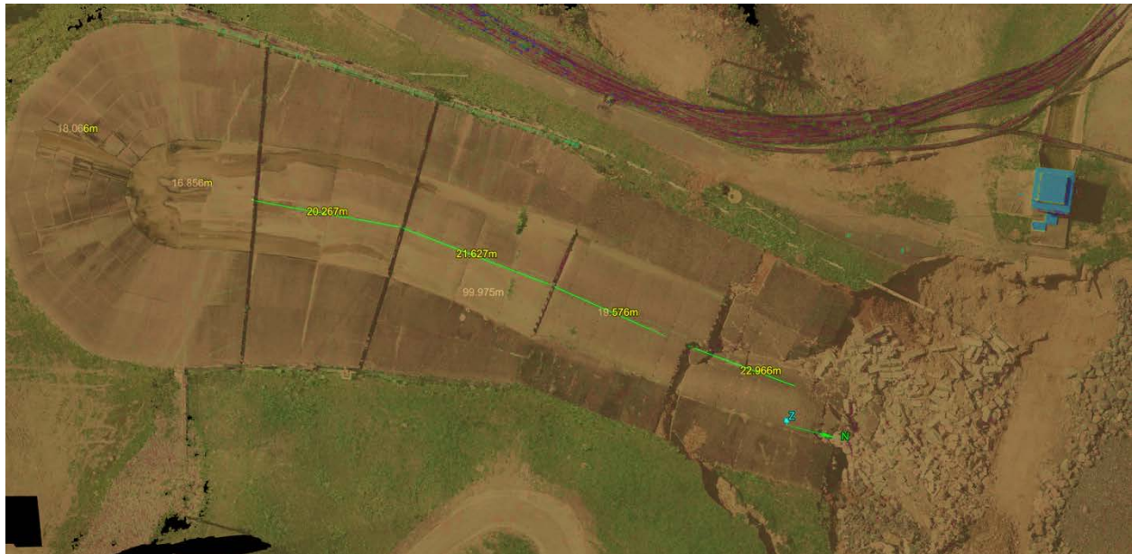
Figure G-2: Hybrid SFM-TLS model of Guajataca spillway with length measurements of individual panel segments.
