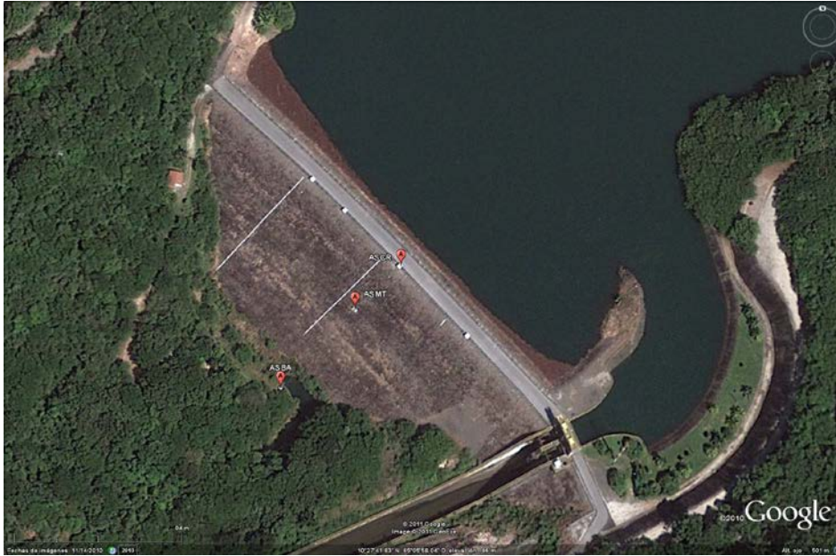
Fig. 6.2 - Aerial photograph of Sandillal dam showing the accelerometer locations in red. (10.46173° N 85.09958° W).
