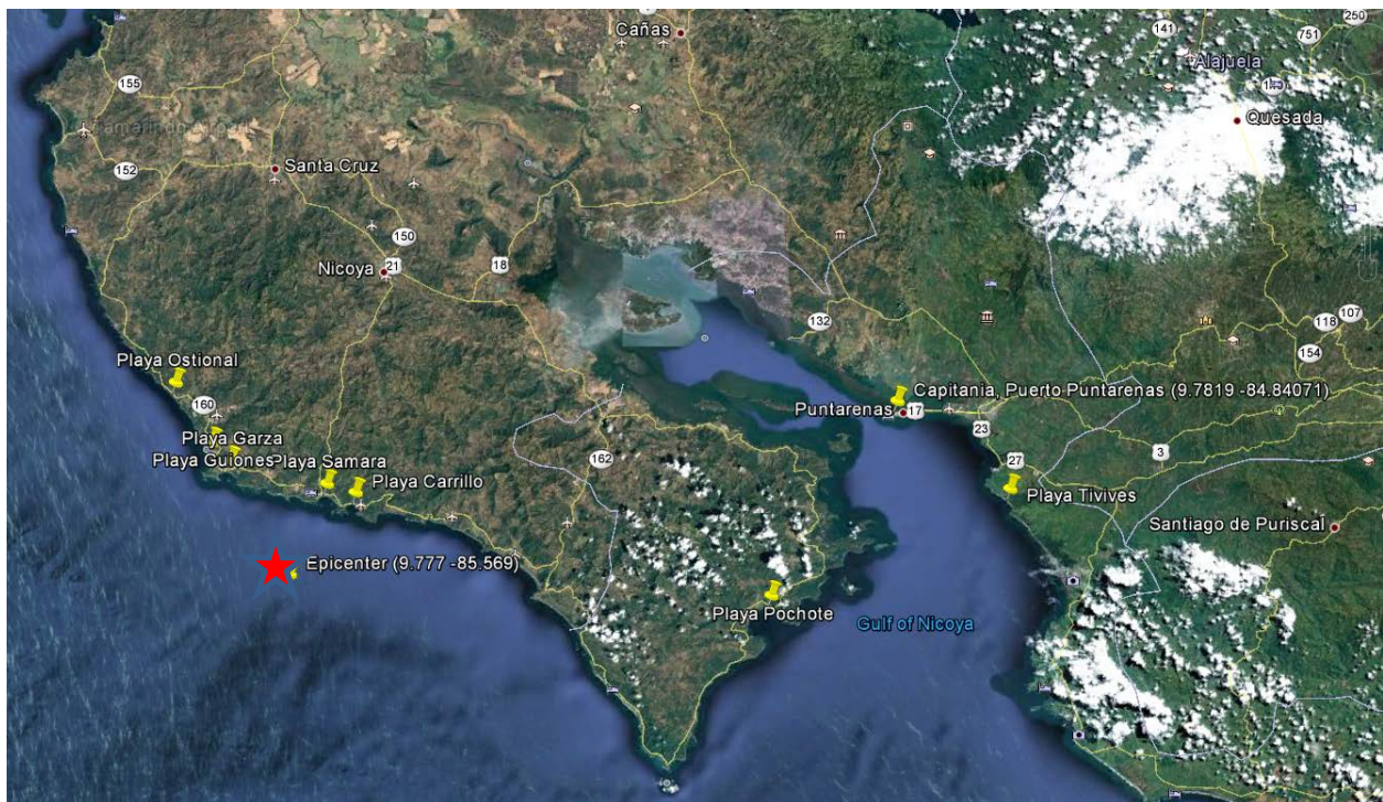
Fig. 2.2 - Google earth map of Costa Rica showing location where liquefaction features were observed during the 2012 Samara earthquake.
