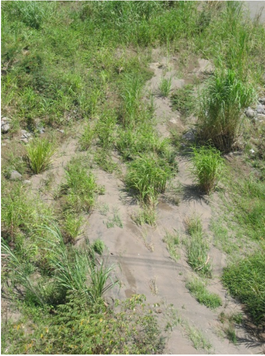
Fig. 4.7 - Ejecta and sand runoff adjacent to the subsided sand boil (9.99676° N 84.69442° W).
