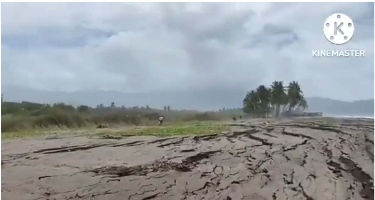
Figure 46. Lateral spreading in beach deposits near Coahuayana, Michoacan immediately after the earthquake (Twitter, 2022). These perishable features were eroded by the tide and waves prior to our visit.
