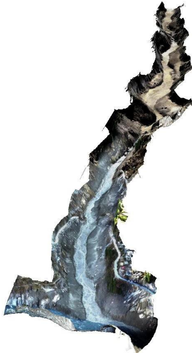
Figure 3.4 Three-dimensional aerial view of the study area-I generated from its DEM draped by the mosaic image. (Dated: February 11th, 2021)
