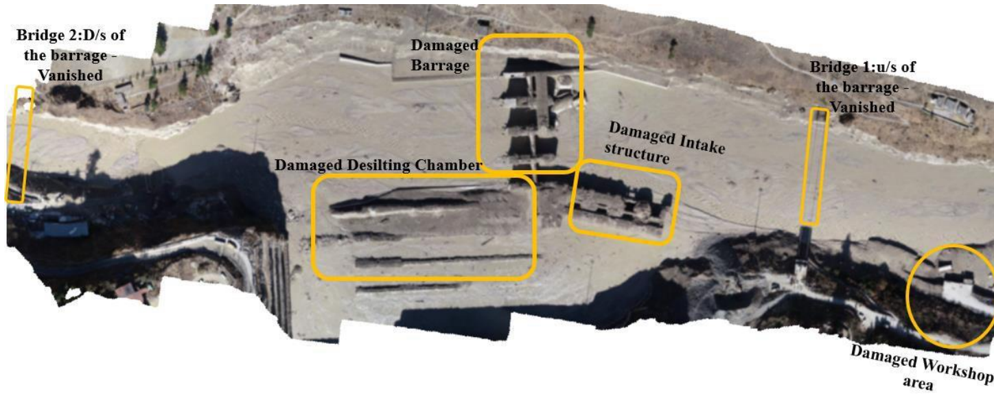
Figure 3.29 Tapovan HEP area (a) pre and (b) post-event orthophoto data showing the collapsed bridges, damaged structures, accumulated boulders, muddy water and, affected barrage gates @ 30°32'7.84"N 79°31'10.71" E
