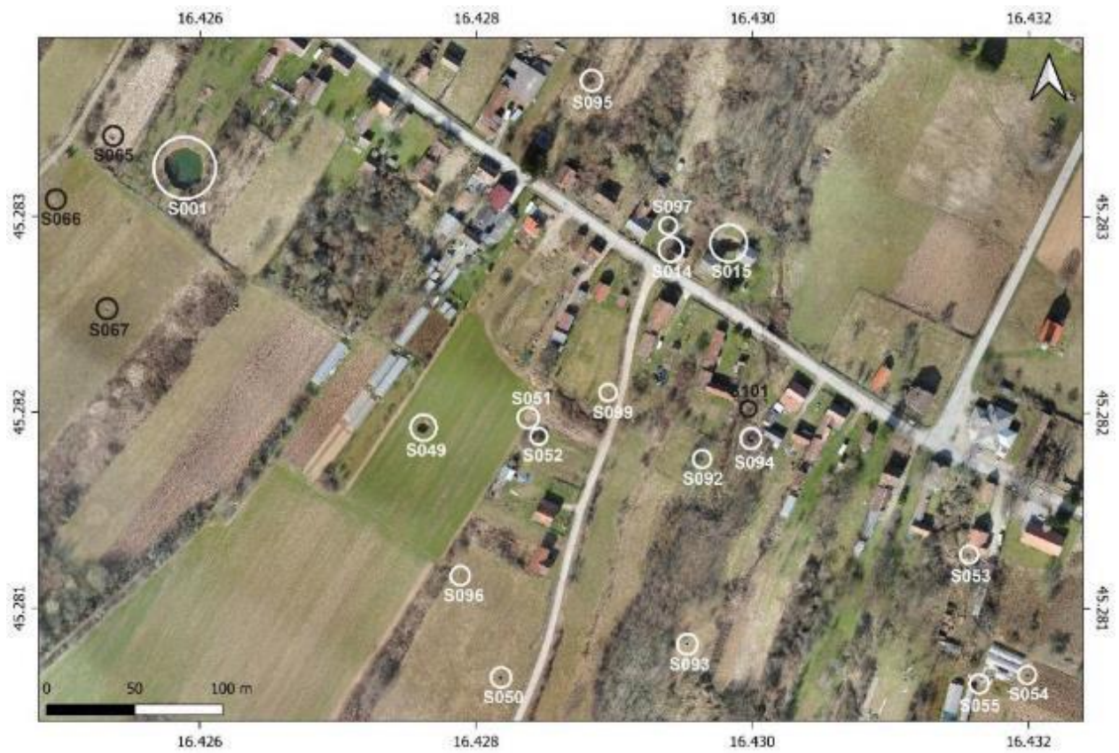
Figure 6.7 Areal image of cover-collapse sinkholes in Mečenčani village (white – new sinkholes opened after M6.4 earthquake, black – fossil sinkholes opened before the Petrinja earthquake sequence). Image by Croatian Geological Survey.
