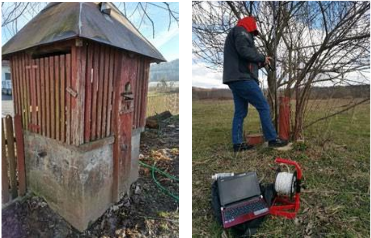
Figure 6.12 a) Typical shallow well in an alluvial aquifer (depth 8 m, shallow well 3 in Table 6.1 ; 45.28154N, 16.43189E), b) Piezometer in a karst aquifer (depth 150 m; 45.29028N, 16.41797E).
