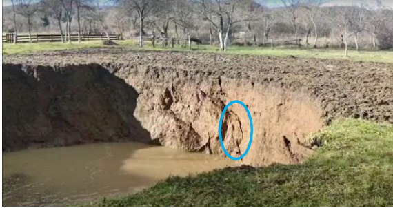
a) The collapse of the edge of a larger unstable clay block.
