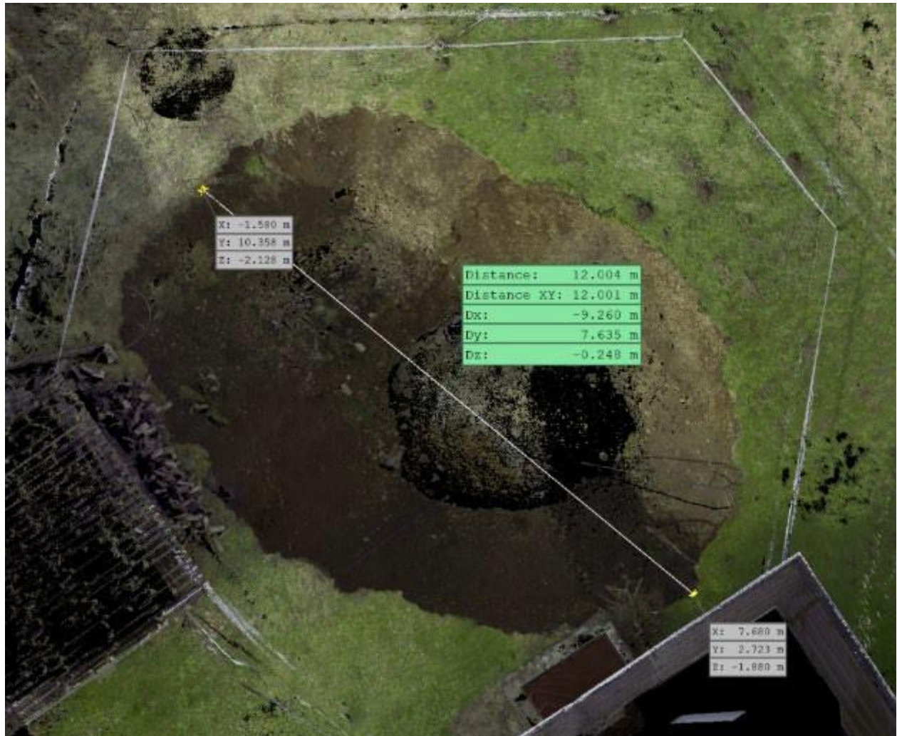
Figure 6.28 Top and bottom diameters from the lidar scan of S015 (45.282859N, 16.429841E).
