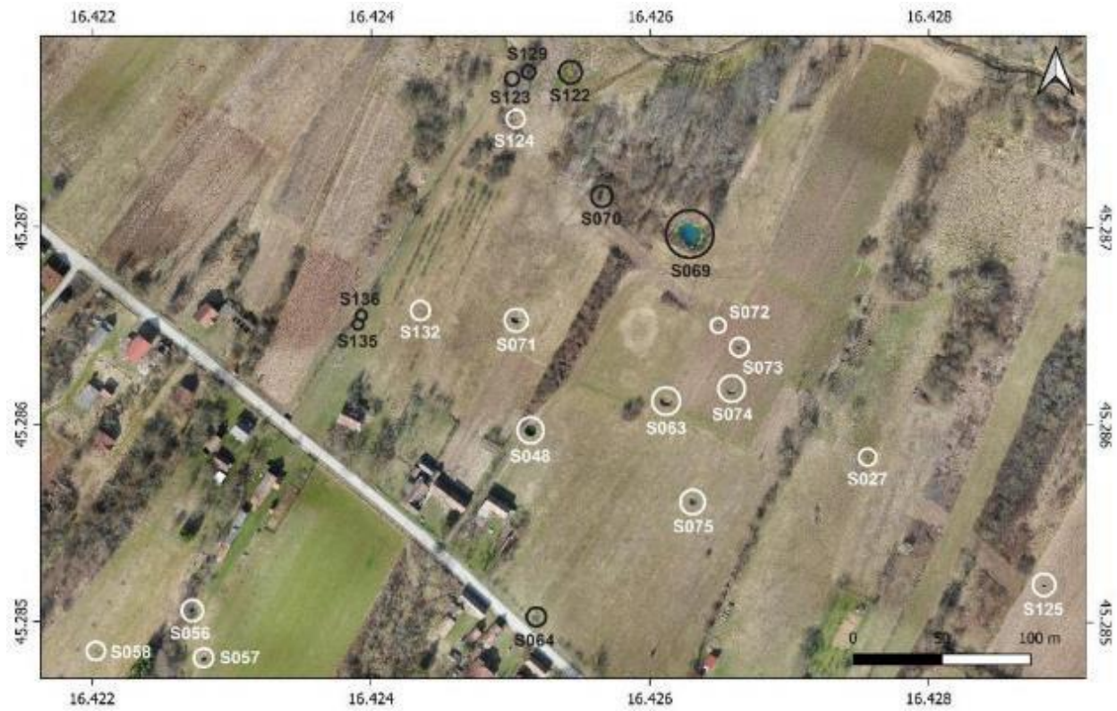
Figure 6.8 Areal image of sinkholes north of Mečenčani village (white – new sinkholes opened after M6.4 earthquake, black – fossil sinkholes opened before the Petrinja earthquake sequence). Image by Croatian Geological Survey.
