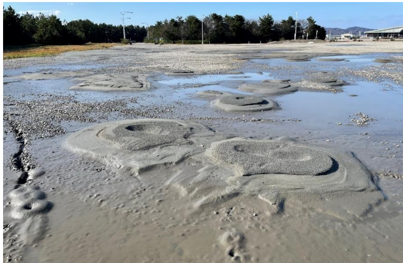
Figure 5.8. Sand eruption site in Shinminato, Toyama Prefecture, Japan (Imizu City, Toyama Prefecture). Lat: 36.78020°, Lon: 137.10301°
