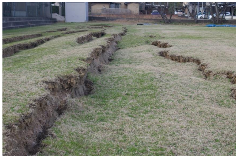
Figure 5.28. Observation of tension cracks at the playground of Nishi Araya elementary school. Lat: 36°40'44.83", Lon: 136°40'2.33"
