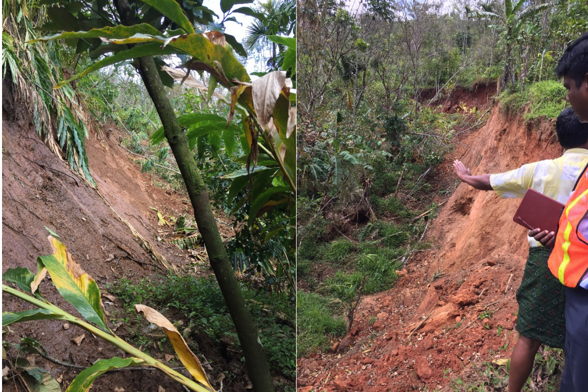
Figure 2.14: Photographs of the main headscarp of the largest landslide in Idukki ( 9.7964191^{\circ}\text{N} ; 77.0682762^{\circ}\text{E} ).
