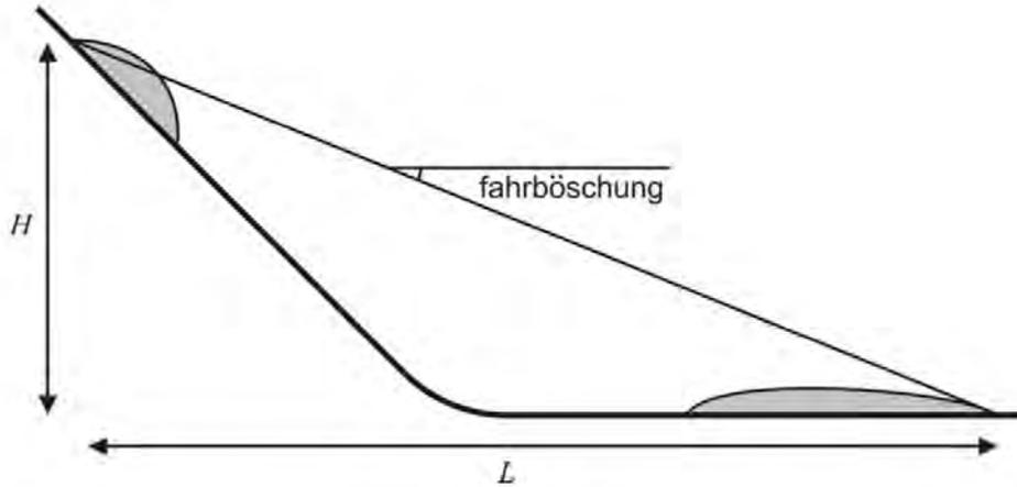
Figure 7.2.1 Definition of angle of reach or fahrböschung (after McDougall, 2006).
