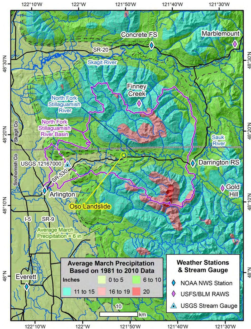
Figure 3.1.1 Map of the Oso Landslide region showing locations of selected weather stations and a stream gauge. Seven weather stations and a stream gauge with the drainage basin outline of North Fork Stillaguamish River; Base map is NWS GIS data of average March precipitation based on the 30-year interval between 1981 and 2010 (GIS file for State of Washington obtained from <http://datagateway.nrcs.usda.gov/>).
