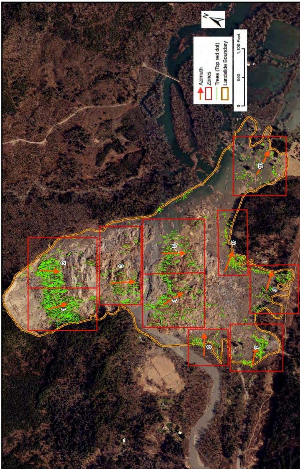
Figure 5.3.2 Areas used for evaluating tree density within landslide boundary
