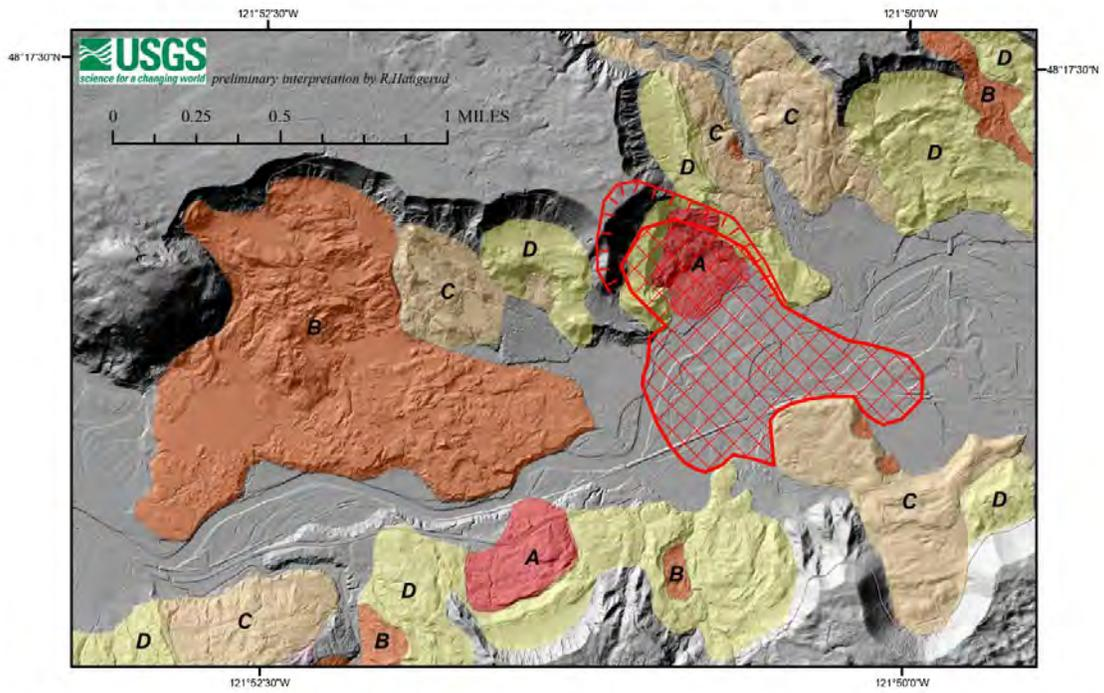
**Figure 2.** Shaded-relief image calculated from the 2013 lidar survey. Colored areas show older landslide deposits, distinguished by their relative age: A, youngest to D, oldest. The red cross-hatched area marks the approximate extent of deposits from the March 22, 2014, landslide.
