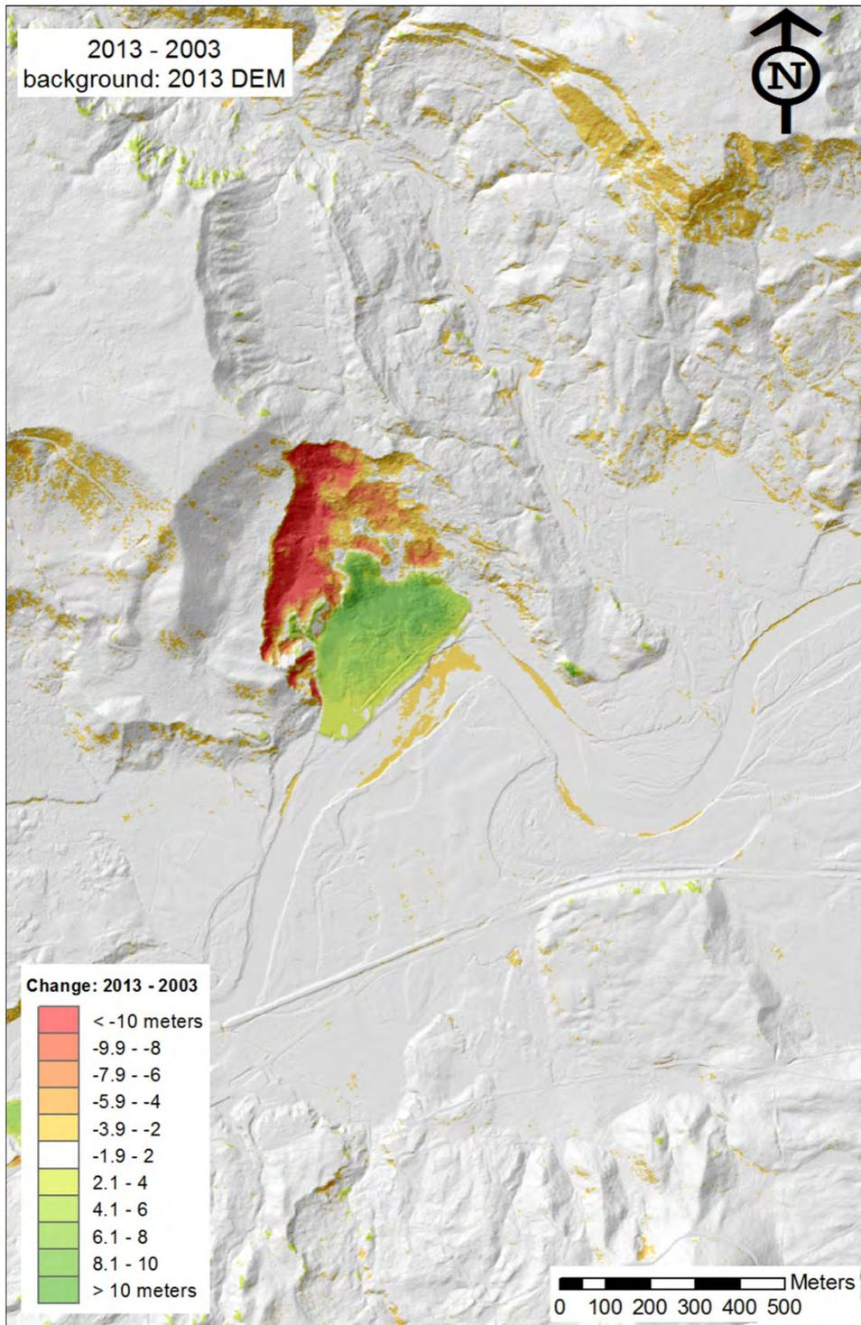
Figure 4.1.5: Elevation differences between 2013 and 2003 lidar data sets. Color keyed to vertical change, with red hues representing decrease in elevation (net erosion), and green hues representing increase in elevation (net deposition).
