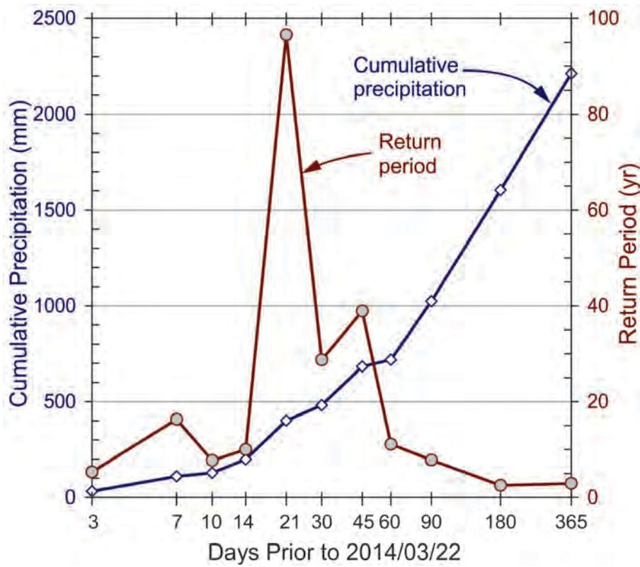
Figure 3.2.1 Cumulative precipitation preceding March 22, 2014, and associated return period at the Darrington Ranger Station gauge. Plotted from values presented in Cao et al. (2014).
