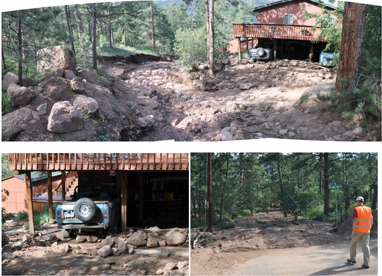
Figure 3.4.11. Flood effects near the apex of the alluvial fan at Cascade. Top: panoramic view looking southwest at Unnamed Creek 3 from Pyramid Mountain Road. Bottom left: detail of carport area in top photo showing boulders on the concrete slab. Bottom right: view looking northeast up Unnamed Creek 3 from Pyramid Mountain Road; absence of boulders is conspicuous. Views from 38.8996° N, -104.9635° W, approximate elevation 7599 ft.
