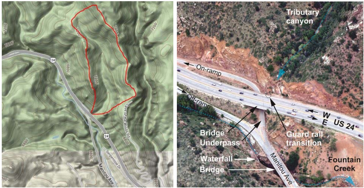
Figure 3.2.15. Tributary canyon draining onto cut slope on US 24 westbound shoulder at bridge abutment with dark water flood discharge captured in YouTube video by MMaksimow (Figure 3.2.14. Left: shaded relief topographic map from Google Maps with drainage basin outlined. Right: aerial oblique photograph taken August 17, 2013, showing details of the US 24 overpass of Manitou Avenue.
