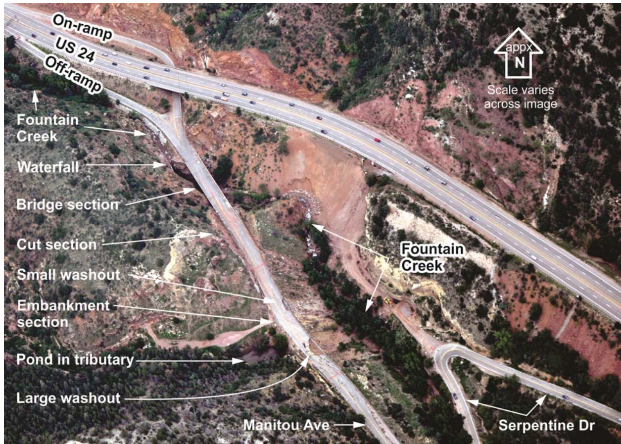
Figure 3.2.18. Aerial oblique photo of Manitou Avenue showing selected features, including two washout areas. Aerial oblique photograph taken August 17, 2013, as part of the GEER reconnaissance.
