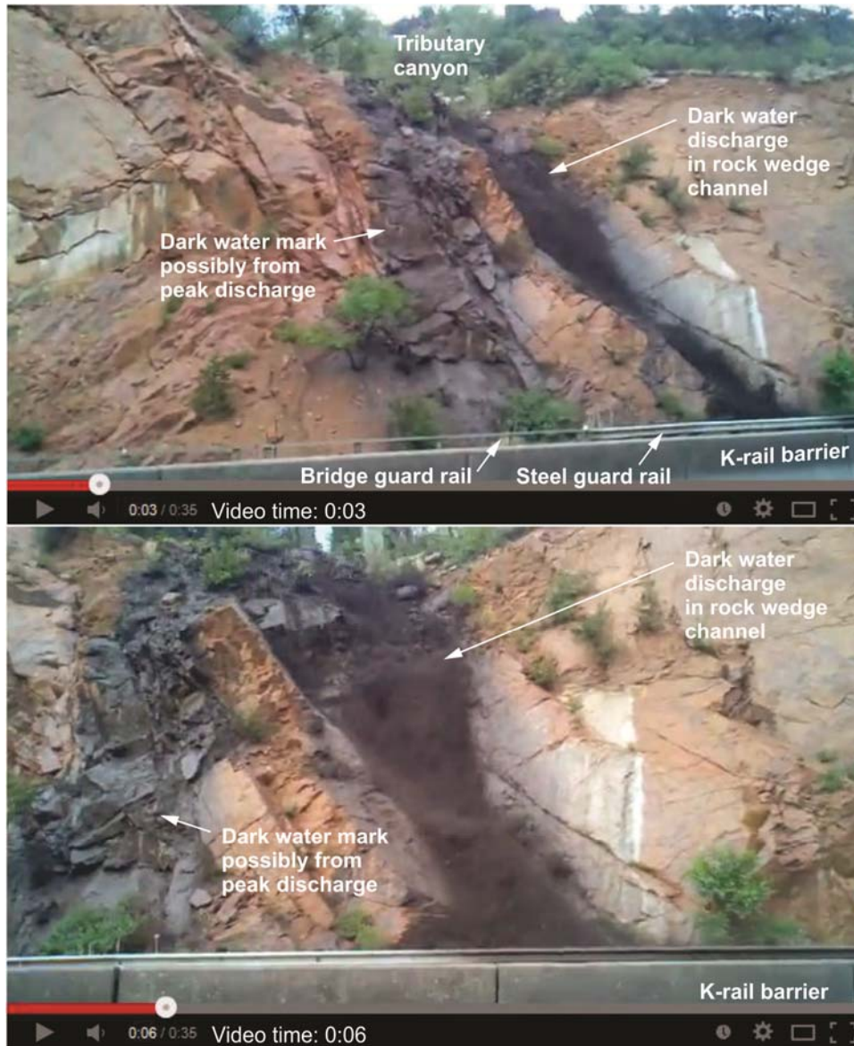
Figure 3.2.14. Screenshots from YouTube video by MMaksimow at two times during its 0:35 duration. Upper (video time 0:03): dark water discharge over cut slope on westbound US 24 shoulder just southeast of overpass on Manitou Avenue where it becomes the westbound on-ramp; view toward the northeast over K-rail barrier from eastbound lanes of US 24 showing the transition from steel guard rail to bridge guard rail. Lower (video time 0:06): same view as upper screenshot with rock wedge more clearly visible.
