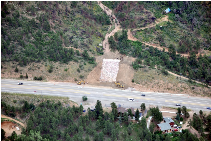
Figure 3.4.13. Aerial oblique views of the mouth of Unnamed Creek 6 located about 1.5 miles northwest of Cascade. Inclined rectangle is a partially grouted riprap panel that was under construction at the time of the GEER reconnaissance (August 17, 2013). The toe of the riprap is located at 38.9123° N, -104.9769° W, approximate elevation 7552 ft.
