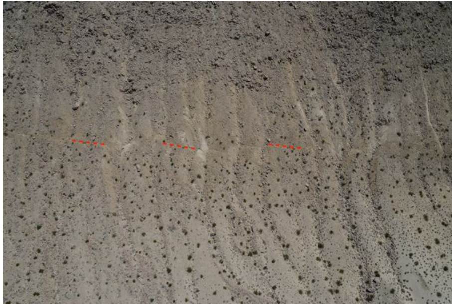
Figure 8. A series of nearly parallel and sharply incised small drainage gullies occur along a NW-SE oriented ridge line that lies from 1 km to 3 km southeast of the offset access road shown in Fig. 7. The roughly twenty such gullies shown in this photo are referred to as the “offset gullies”. The short dashed red line segments indicate the location of the mainshock fault surface rupture, which forms a bench as the fault cuts across this hillside, nearly perpendicular to these gullies. With high-resolution topography from the air photos already collected, and potentially from the airborne lidar in the future, geologists expect to be able to precisely measure fault slip variation along this section of the fault. Slip is known to diminish from approx. 1.8 m at the abandoned railroad tracks down to less than one meter at the SE end of the ridge where these gullies were found. So, it is expected that these gullies will afford a way to quantify the reduction in slip from NW to SE along this 2 km long section of the fault.
