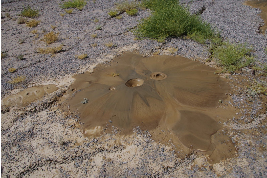
Figure 31. Sand boil near margin of Searles Lake in Trona. Photo by Scott Brandenburg, (35.7573, -117.3776).
