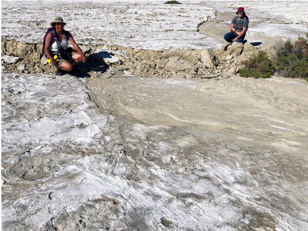
Figure 6. A 4.20 m right-lateral offset is measured by Belle Philobosian (USGS) and Kelly Blake (NAWSCL Geothermal Program Office) on the dry lake bed (playa) surface of China Lake. The channel margin sharply demarcates the salt-crusted white surface of the pre-incisional dry lake bed surface from the fresh fine-grained deposits in the wide flat channel thalweg. This sharply defined feature provides a reference line that allows measuring this displacement vector with unusually small errors of approx. \pm 5 cm. This is considered the maximum offset measurement obtained as of this writing (Credit: photo by Brian Olson, CGS).
