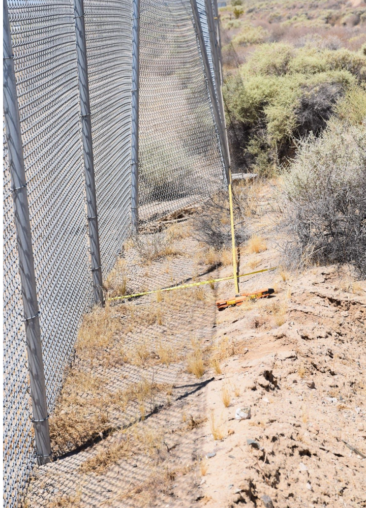
Figure 9. Offset fence line at southern Salt Wells Valley, just north of highway 178. The fence offset is 70 \pm 5 cm right-lateral sense. (photo by Jason R. Patton, CGS; Lat./Long. 35.6495, -117.4828)
