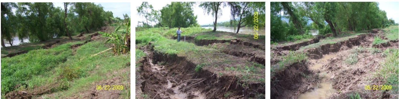
Figure 9 – Multiple views of severe lateral spreading between levees and river [06/22/2009, 10:25AM, N15.391266, W87.845191].
