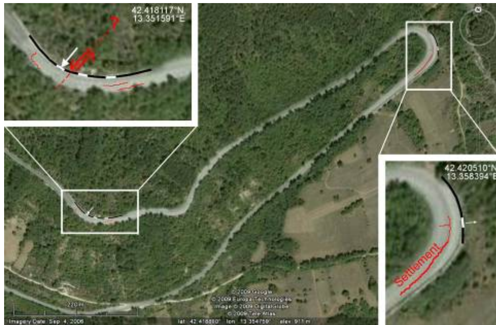
Figure 6.16. Locations of observed pavement cracking and associated retaining wall failures.
