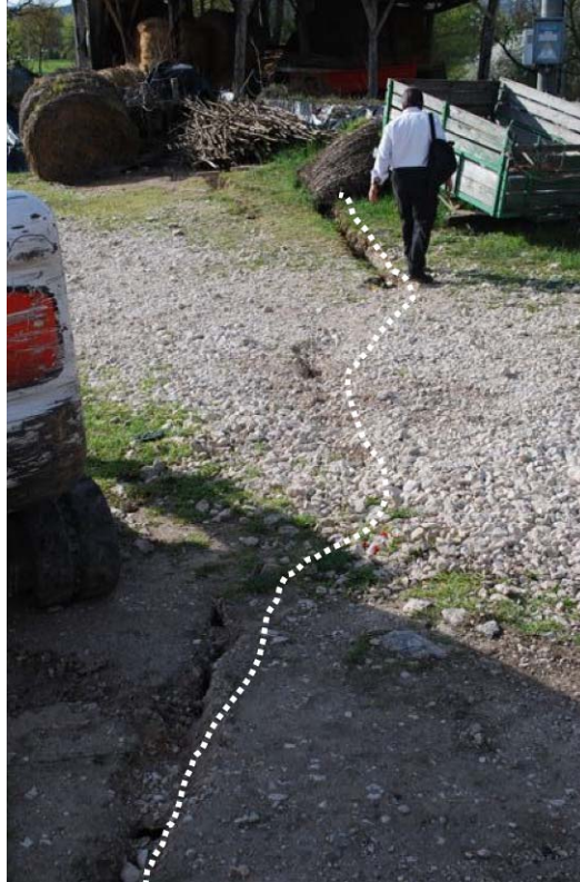
Figure 5.32. Ground cracks up to 1.0 m deep, 20 m long, and with maximum 0.15 cm vertical displacement (down-dropped toward river) developed directly adjacent to bridge abutment (42.324N, 13.478E).
