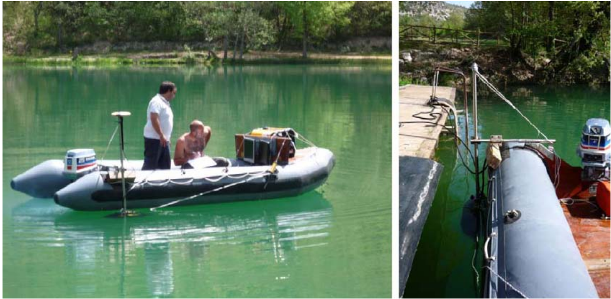
Figure 5.61. Rubber boat equipped with the 8101 multibeam system.
