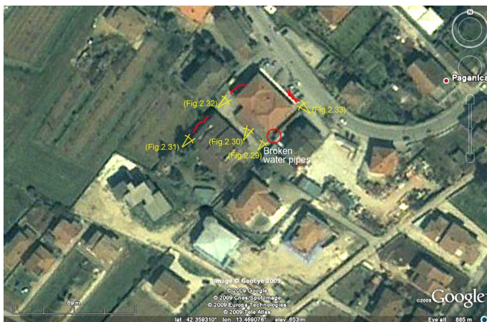
Figure 2.28 Plan view of Paganica site with marked positions of ground fissures, paved walkway cracks and broken water pipes. Directions of photo shots are indicated by yellow signs.
