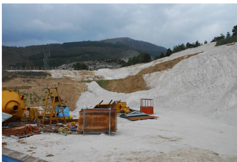
Figure 5.17. Quarry in Cataclasite with near vertical slopes segments up to approximately 15 m high, located northeast of Colle (42.435N, 13.330E).
