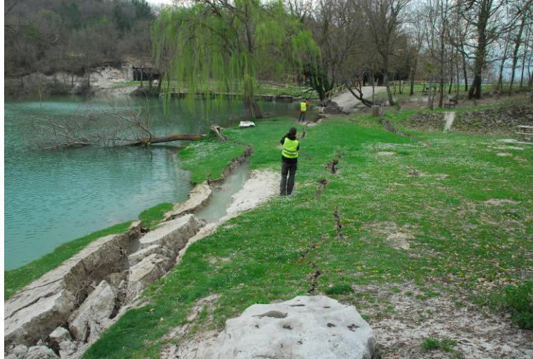
Figure 5.47. Ground cracks along the northwest perimeter of Lake Sinizzo (42.291N, E13.576).
