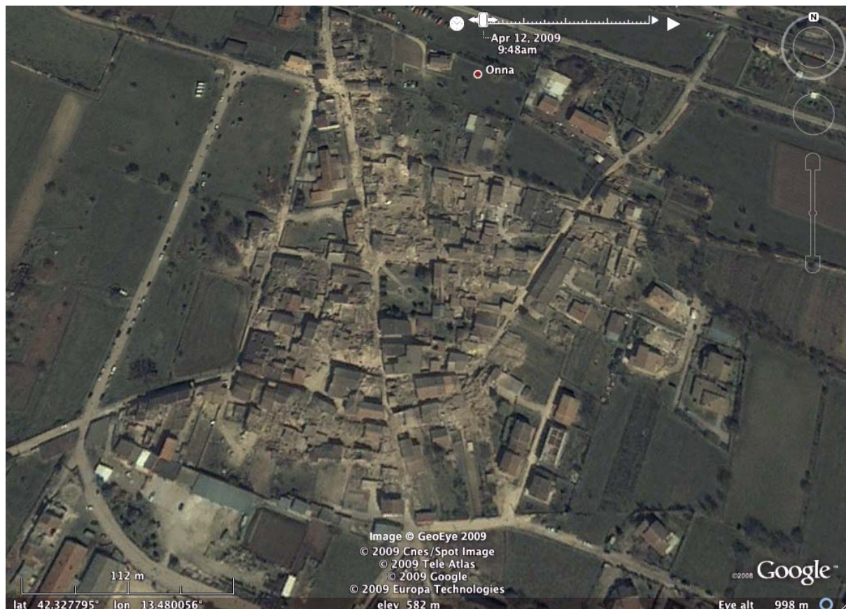
Figure 4.11. The village of Onda suffered D4—D5 damage in most of the unreinforced masonry structures. Reinforced concrete structures at the margins of the village performed well with only minor damage (D0-D2).
