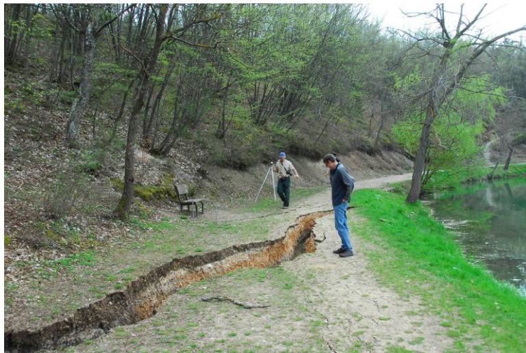
Figure 5.48. Ground cracks along the eastern perimeter of Lake Sinizzo (42.291N, E13.576).
