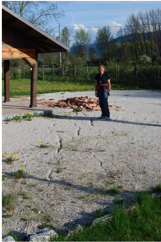
Figure 5.29. Ground fissures developed in alluvial floodplain directly south of central Onna and approximately 150 m from the Aterno River. Orientation of fissures is approximately parallel to the river (42.325N, 13.480E).
