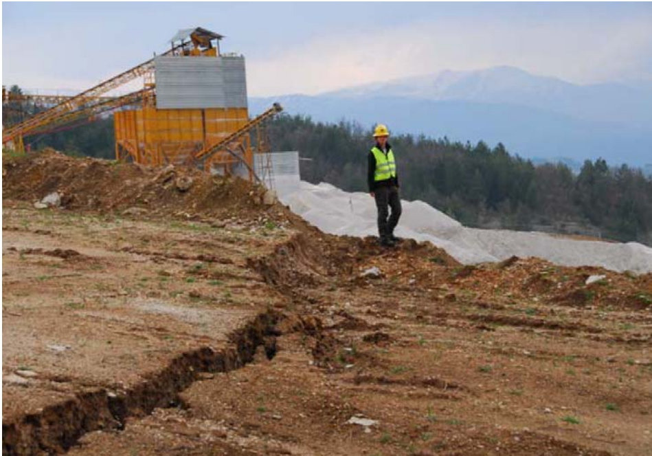
Figure 5.38. Shear failure developed in fill material, with vertical displacement increasing to approximately 40 cm at free slope face (42.435N, 13.330E).
