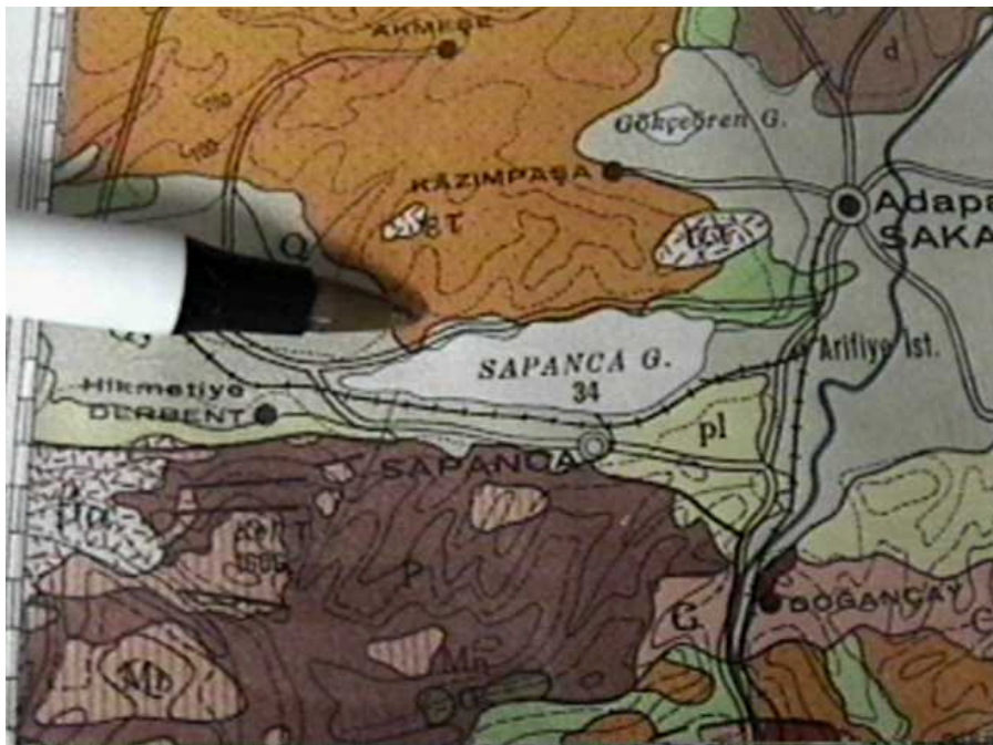
Assumed position of existing landslide north of Sapanca lake. The geological map represents a recent quaternary deposit which could be sliding toward Sapanca lake ( N40^{\circ}44.027' , E30^{\circ}13.275' , 8/27/99, 11:24:52).
