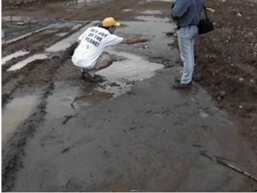
In the open space between the buildings of the Ford plant of Golcuk, a large sand boil erupted and littered the ground surface with silty sand (N40°43.165', E29°50.596', 8/28/99, 15:42:14).
