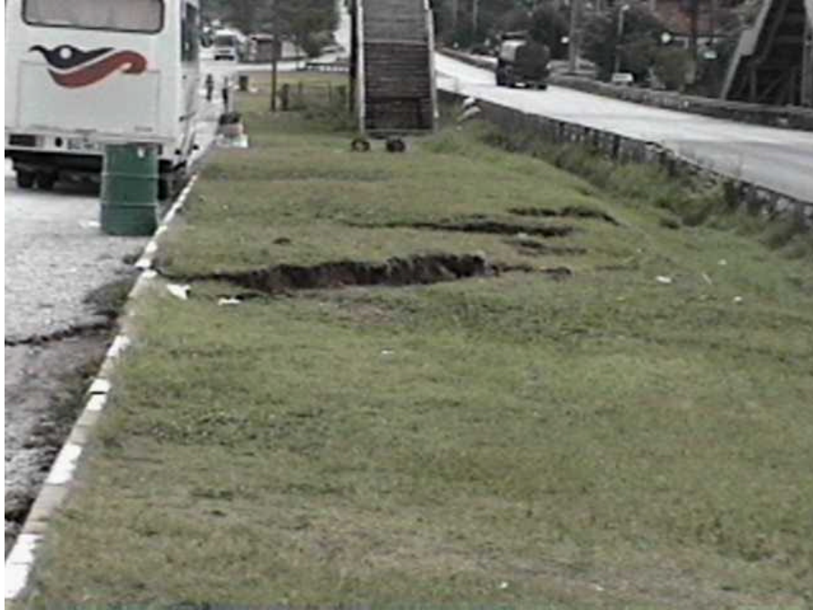
Ground cracks were noticeable from the highway north of Sapanca lake. These ground cracks were attributed to the reactivation of large existing landslides after the earthquake ( N40^{\circ}44.027' , E30^{\circ}13.275' , 8/27/99, 11:24:52).
