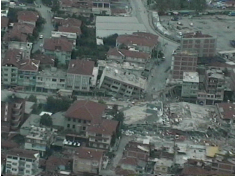
The collapse of buildings was widespread, but not uniform in Adapazari, possibly due to different soil conditions and inconsistent enforcement of building codes (N40°46.329', E30°24.328', 8/24/99, 15:47:42).
