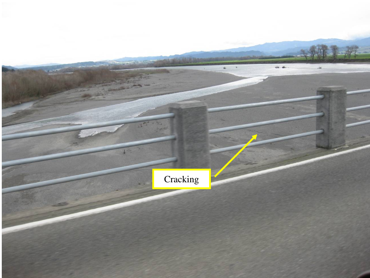
Figure 25 Ground cracking was observed in the Eel River channel near Fernbridge. This gravel bar was inaccessible by foot (channels on either side) and Fernbridge is a narrow two lane bridge without any pullouts, thus, additional information was not able to be collected at this location. (40.613716N; 124.202568W).
