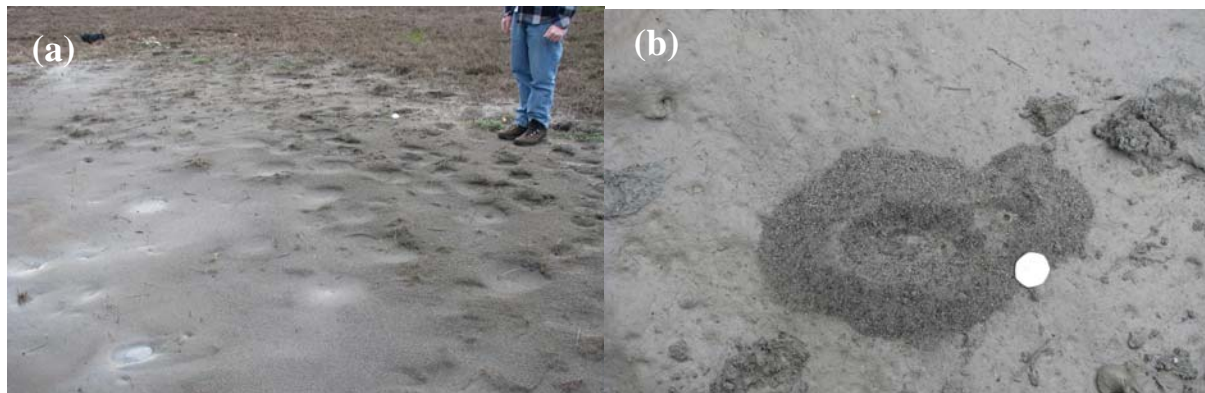
Figure 11 Liquefaction features: remains of sandboils at Centerville Beach (a) and sandboils along the Eel River (b).
