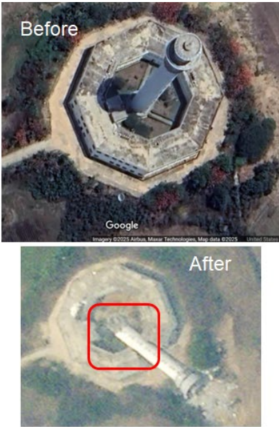
Figure 6.2.7. Collapsed airport control tower of the Nay Pyi Taw airport due to biaxial bending resulting from combined effect of horizontal ground motion components (Source: @heungburma on X ), with aerial imagery of condition before and after earthquake (Sources: before, Airbus, Maxar Technologies; after, Maxar Technologies).
