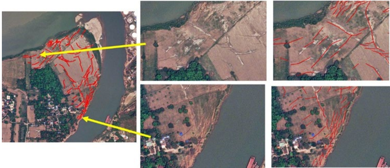
Figure 4.3.1. Mapping of lateral spread features showing differing fissure and ejecta patterns in Area 3. Inset images show magnified views of two subareas. Lateral spread fissures marked in red.
