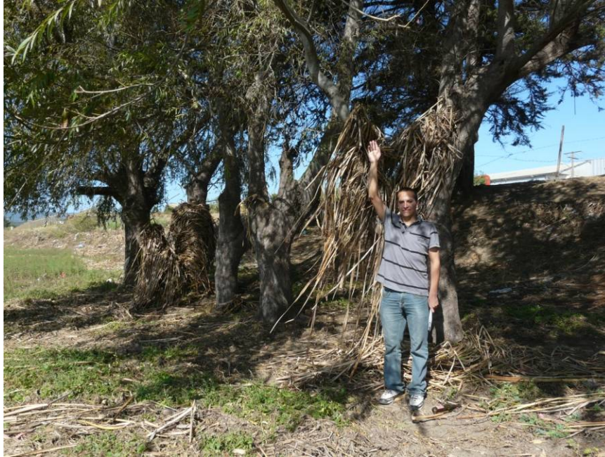
Figure 13.31. Debris suspended in trees along a lagoon north of Pichilemu indicate tsunami flow depths exceed 3 m at this site (S34.385195° W71.999901°, 1619 hrs on 03/14/2010).
