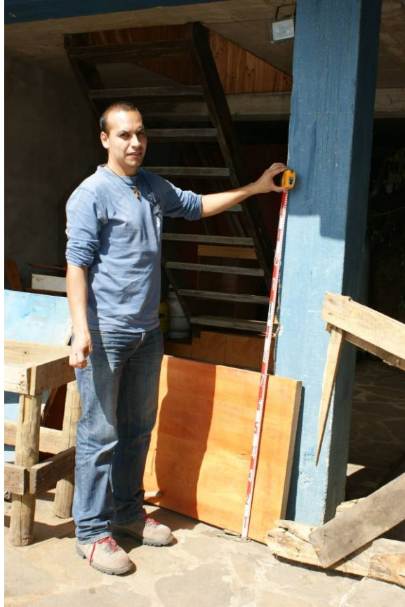
Figure 13.23. On this post inside the first floor of a beach front house in El Torreon, a small community south of Pelluhue, visible lines mark the water height 1.6 m above the ground providing a minimum estimate of the tsunami flow depth at this location (S35.8214°, W72.8215°, ~1556 hrs on 03/17/2010).
