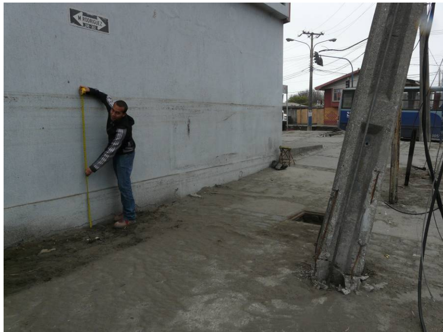
Figure 13.5. Along Avenue Manuel Rodriguez in Talcahuano, the tsunami reached minimum flow depths of 1.6 m (S36.725249° W73.106313°, 1215 hrs on 03/16/2010).
