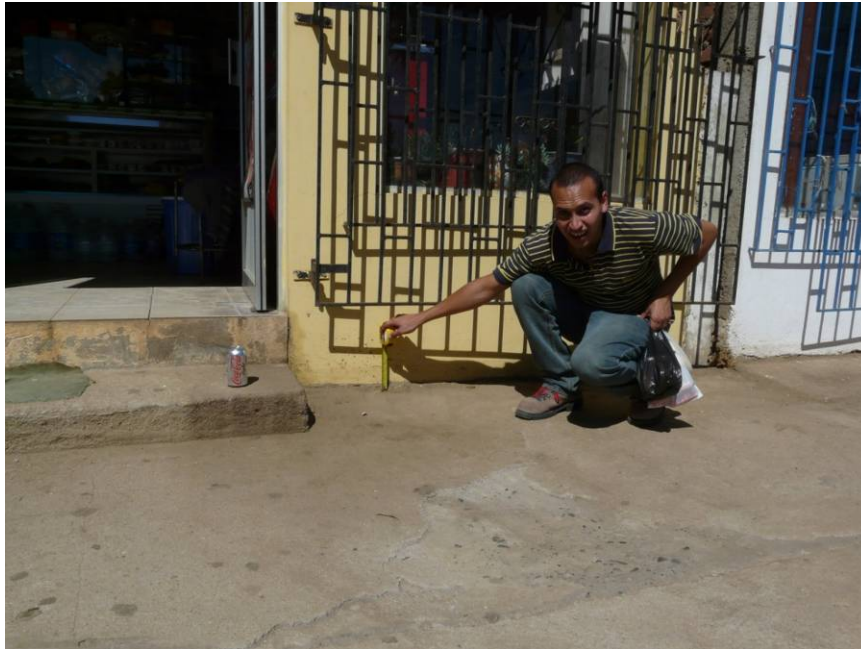
Figure 13.29. Tsunami flow depths at the east end of Bucalemu reached 0.1 m or less near the landward limit of tsunami inundation (S34.642586° W72.037371°, 1228 hrs on 03/15/2010).
