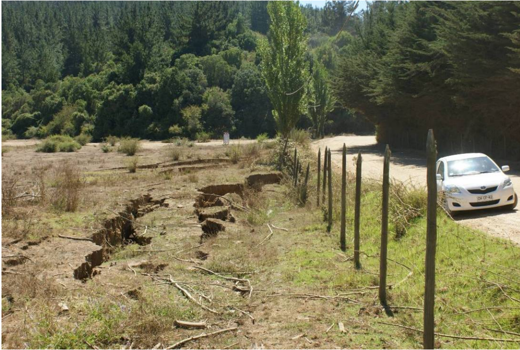
Figure 14.12. Lago Vichuquen,. Lateral spreading on the inland side of the lakefront road. (S34.39097°, W72.077815°; 12:46 hours on 3/15/2010)
