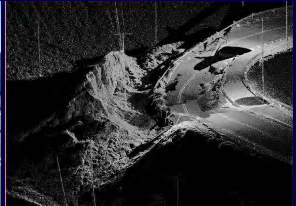
Optical & LIDAR Images: failed embankment on Ruta 5 (2010 Chile EQ - Kayen in Bray & Frost 2010)
