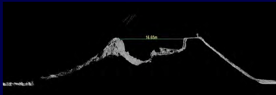
Optical & LIDAR Images: failed embankment on Ruta 5 (2010 Chile EQ - Kayen in Bray & Frost 2010)
