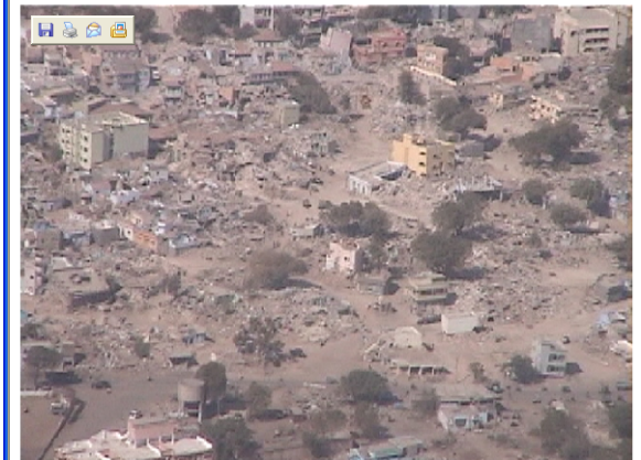
Figure 31. Very few masonry buildings were left standing 2 km to the Southeast of the Anjar (2/12/01 11:14:50 AM, N23.10079 E70.05062).
